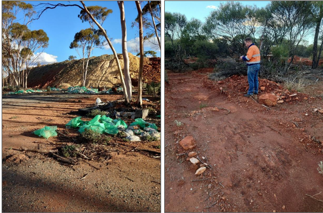
Figure 5.13: Remnants of RC/RAB footprint surrounding historical workings and track clearing for nugget gold detection along shears at Yarbu
